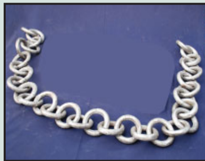
Cast Chain (ASTM A-351 HK 40)
