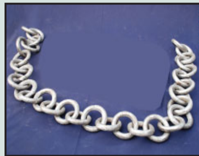
Cast Chain (ASTM A-351 HK 40)
